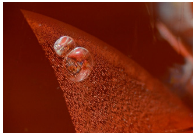
Heated orange sapphire revealing two characteristic disc-like atoll structures extending from fine fluid tubes. Photo: M.S. Krzemnicki, SSEF
