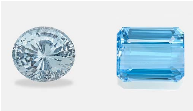
Left: Untreated light blue topaz (natural colour) and right: irradiated blue topaz (treated colour). Photo: SSEF
